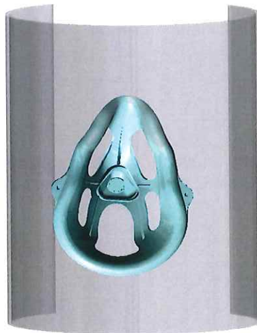
Figure 1-Mask Mounted on Cylindrical Surface
